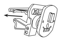
Step 3. Adjust the support leg vertically until it rests firmly along the bottom of the vent or dash surface below the vent. It will need to support the weight of the cradle and device.
